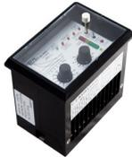
These relays were designed to accommodate a wide range of mounting options. Current range detection is 5 to 550 A but protection features vary between models. Some include a 4 to 20 mA output. Variable user-selected thermal curves 2.5
